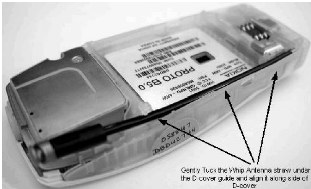
Figure 5: Properly installed whip antenna
